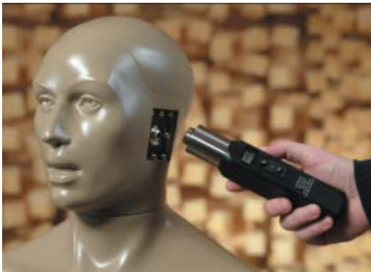
Figure 11. Using a pistonphone to calibrate a HATS ear simulator microphone.
