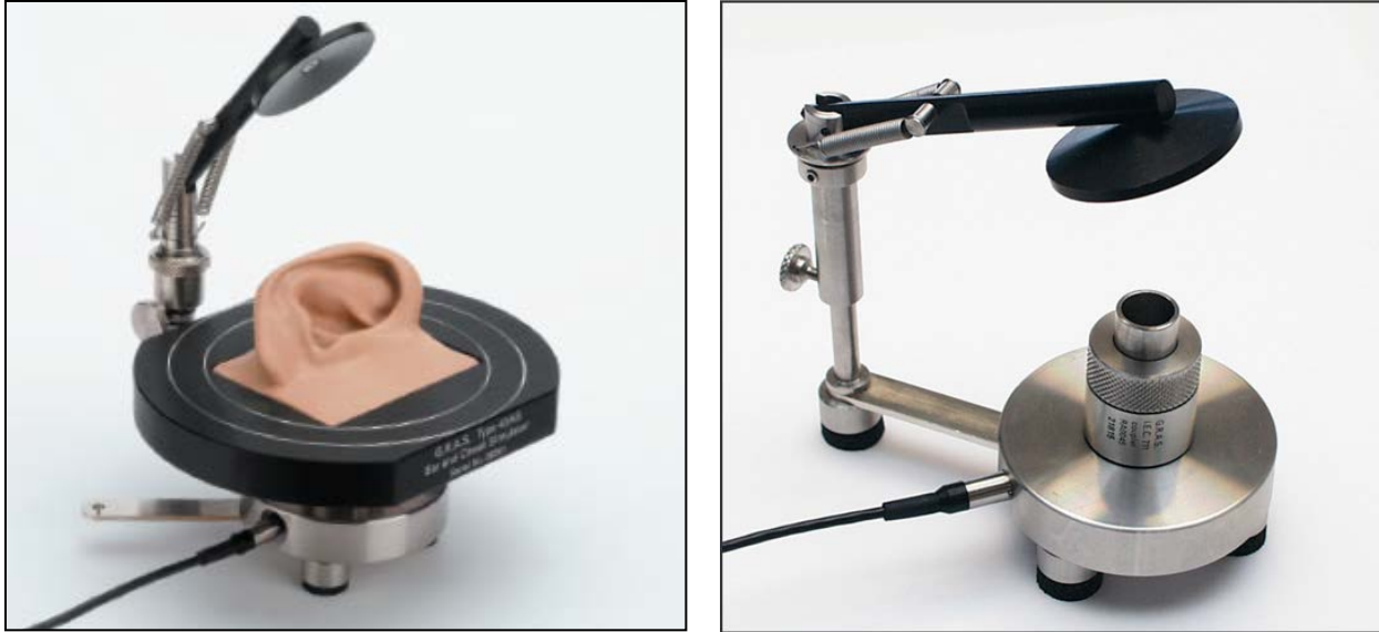
Figure 7. G.R.A.S. Type 43AG Ear and Cheek Simulator (left) and Type 43AC Artificial Ear.
